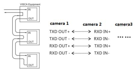
The RS232 cascade connection way is almost the same as that of RS422. The output of camera 1 is connected with the input of camera 2, the output of camera 2 is connected with the input of camera 3, and so on so forth.
