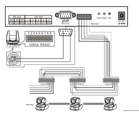
1.control output:connect camera RS485+ with keyboard Ta, RS485- with Tb.
